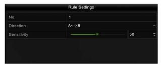
Figure 9-6 Set Line Crossing Detection Rules
