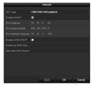
Figure 11-26 Network Parameters Configuration
