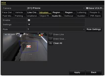
Figure 9-9 Draw Area for Intrusion Detection
