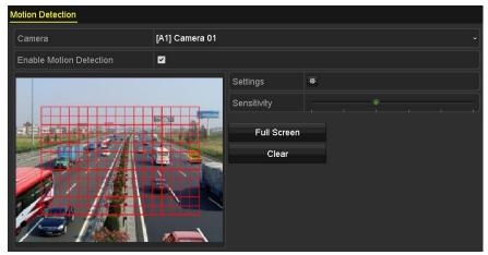
Figure 8-2 Set Detection Area and Sensitivity
