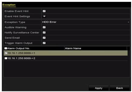
Figure 12-26 Configure HDD Error Alarm
