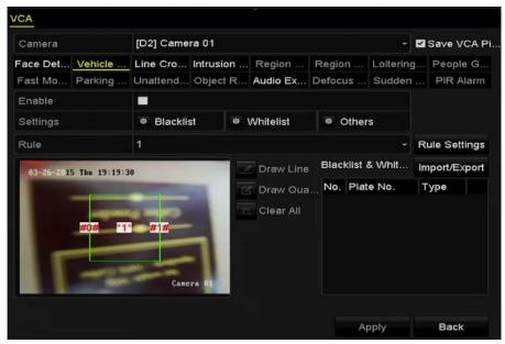
Figure 9-4 Set Vehicle Detection
