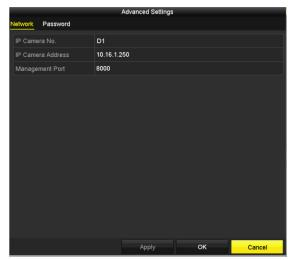
Figure 2-42 Network Configuration of the Camera
