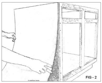
the edge. On larger surfaces you may want to lay down some separator strips or dowels to prevent the veneer from making contact until you are properly positioned. Again, start in the center and begin removing the strips from the center out applying pressure as you work outward. Now that the veneer is
