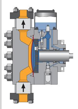
Principle of diaphragm pump head
