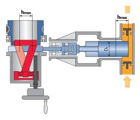
Principle of a flow rate adjustment
