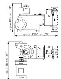
Weight according to equipment (without motor) approx. 515 - 680 kg (1135-1500 lbs.)
