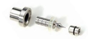
C60 Series valves feature a seal-less diaphragm with a tapered plunger, making the valves ideal for high-pressure requirements and handling dirty fluids.
